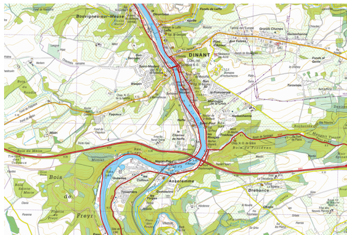
Figure 16.2: The topographical map of Dinant displays elevation by drawing contour lines, along which the elevation is constant.
